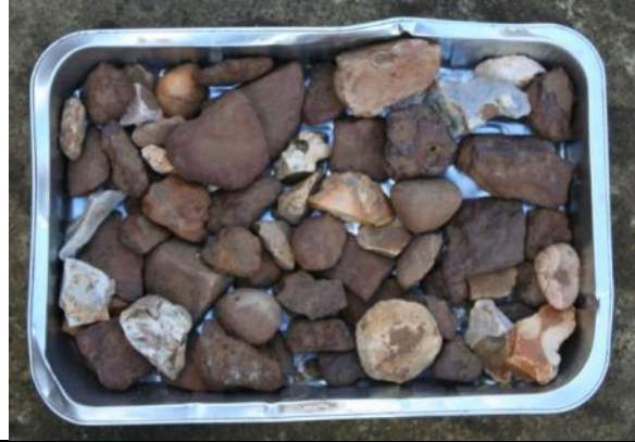
Some subrounded > 2cm stone but significantly more 2mm-2cm stone.
